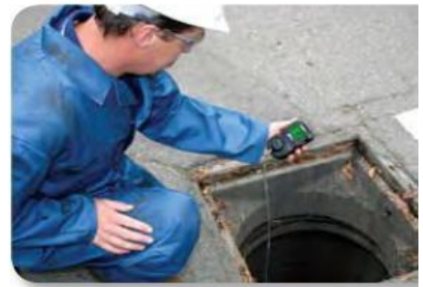
QRAEII being used with built-in pump for a confined space entry
